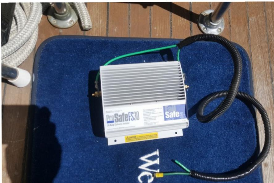
**Lower left:** galvanic isolator with 2 ground wires.
